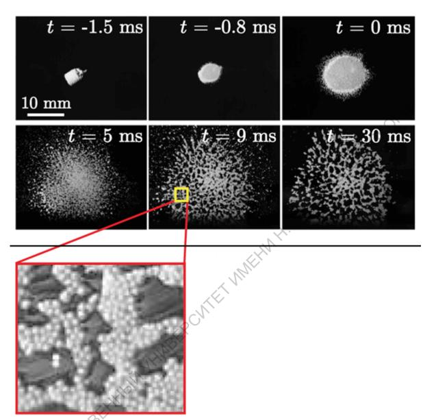
A bottom view of a drop impacting on a glass surface, with t=9ms showing the way the particles spread out and create a lace like structure.
