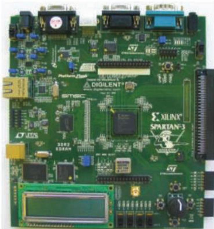
ПЛИС Xilinx Spartan-3AN FPGA Starter Kit Board
