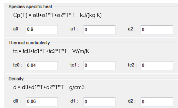
Fig. 3 - Properties of heat insulation
