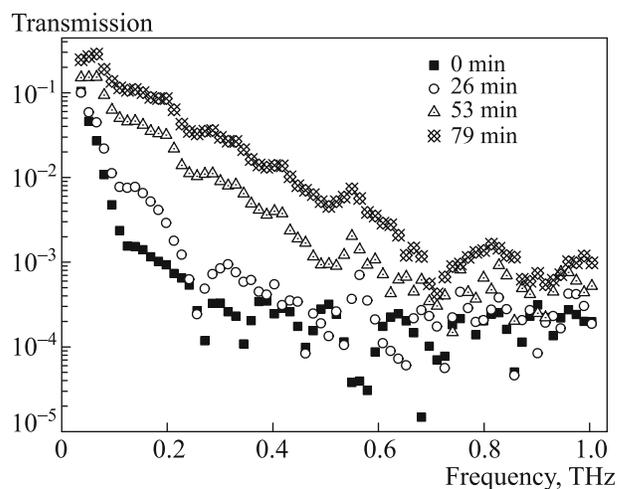
Fig. 4. Transmission spectra of pig muscular tissue affected by glycerol.
