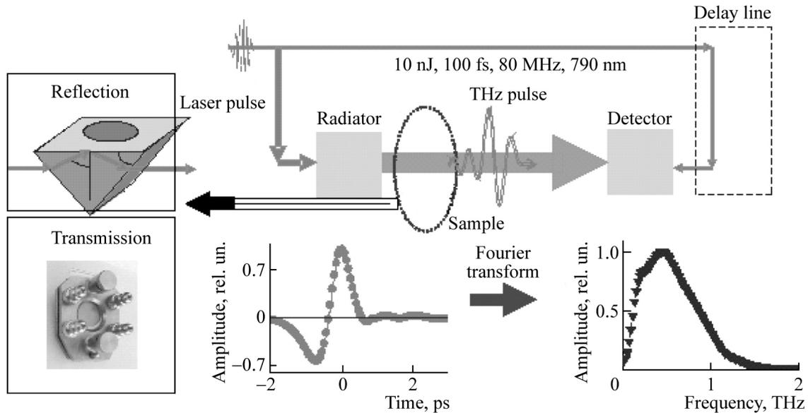
**Fig. 1.** Schematic of a time-domain THz spectrometer. A silicon prism and a metal mounting with polystyrene windows are used in the reflection and transmission geometries, respectively.
