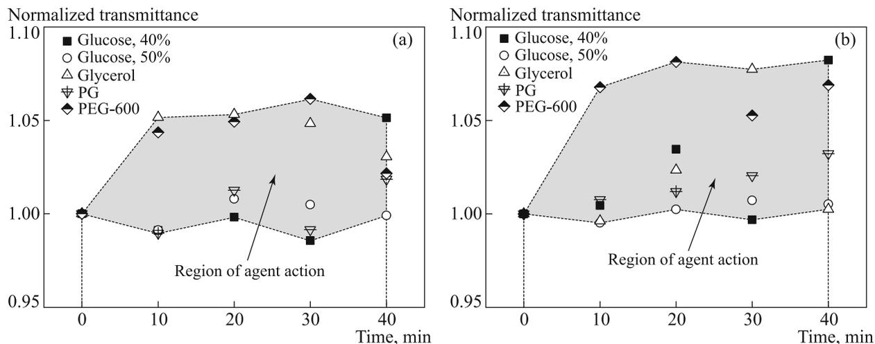
**Fig. 7.** Time dependences of the normalized transmittance of (a) healthy skin and (b) tissue tumor affected by different agents, measured at a frequency of 20 THz.
