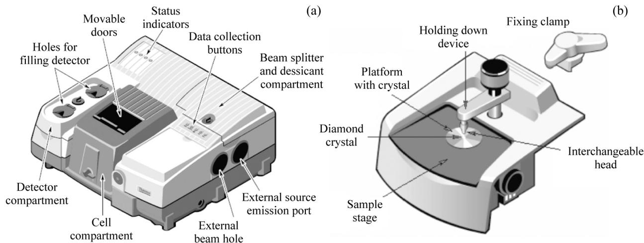
Fig. 2. Experimental setup: (a) Nicolet 6700 Fourier spectrometer and (b) Smart iTR FTIR attachment.
