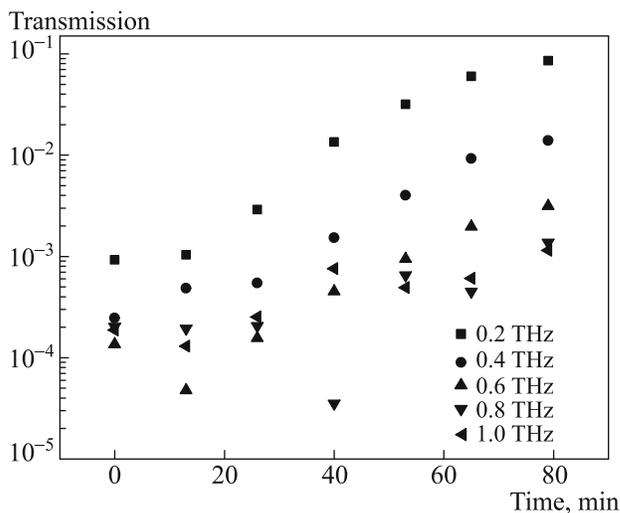
Fig. 5. Kinetics of change in the transmission of pig muscular tissue affected by glycerol at different frequencies.
